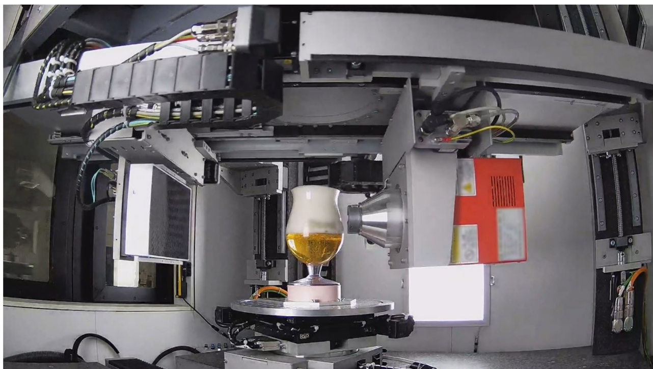
▲ Fig. 1: Delicate beer foam sample mounted inside the DynaTOM.
